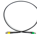
SP-24292-FM24LP / SP-24292-FM36LP / SP-24292-FM48LP Frequency Range: 40 GHz Configuration: 2.4mm female to 2.92mm male Length: 24" / 36" / 48"
